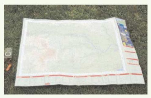
Map orientation using a compass: the map, which may be marked along its north edge with a series of north-pointing arrows, is placed on the ground alongside the compass and adjusted until the compass needle and the arrows are parallel and pointing in the same direction. The variation between magnetic north and true north may be ignored in the primary school.
