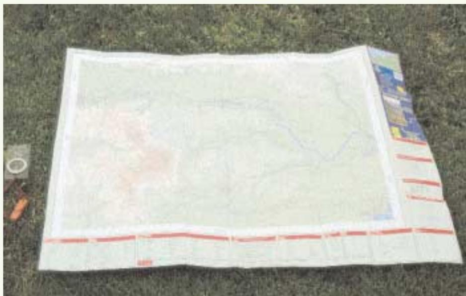
Map orientation using a compass: the map, which may be marked along its north edge with a series of north-pointing arrows, is placed on the ground alongside the compass and adjusted until the compass needle and the arrows are parallel and pointing in the same direction. The variation between magnetic north and true north may be ignored in the primary school.
