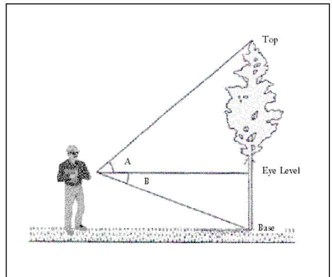
Use trigonometry to calculate the height of the tree.
