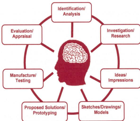
Simplified Diagram of a Design Process
